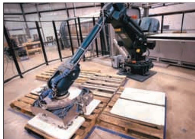
A robotic arm uses suction cups to load dehumidifier panels onto crates after the pieces were cut from a large sheet.
